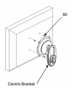
Figure 2. Flush Mount Centris Bracket to Display
